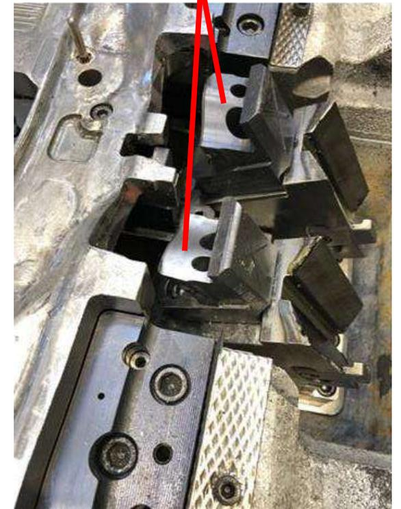
Light damage after 190 100 pcs, there will be re-sharpening and further use of the tool.
