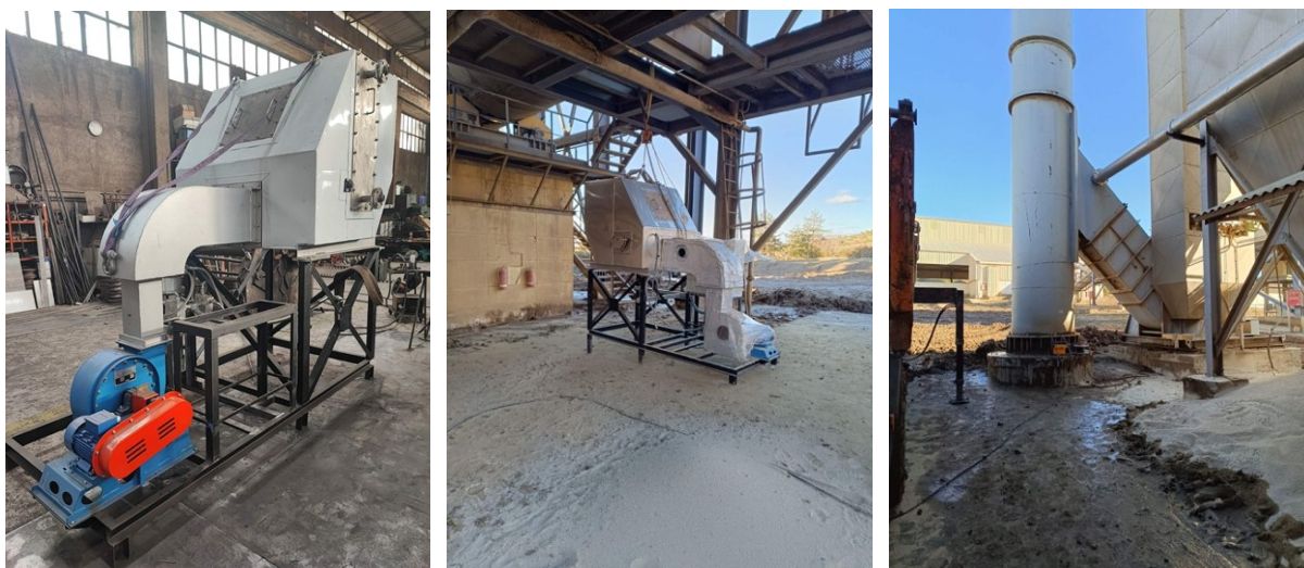
Figure 2: The custom-designed heat exchanger system, developed in Athens and installed in Grevena, capable of processing 1,800 kg/h of waste gas flow. This innovative unit demonstrates efficient heat recovery from the plant's exhaust stream, marking a significant step forward in industrial energy efficiency.
